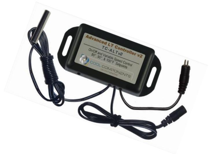
For each Mode, the fan/s will turn on at 50% speed and will increase in speed in a linear progression until full speed is reached at ~10°F above the “On” setpoint. As the system cools down the fan/s will slow down in a linear progression and ultimately turn off when the temperature drops ~3°F/2°C below the “On” setpoint. The alarm is set at a fixed 115°F/41°C.
